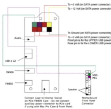
Connections for Hack Pro front panel PCB part number 820-2501-A to Digitec's CA-70500-LE02m-03 motherboard.
