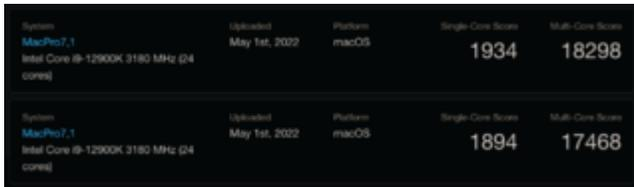
The image shows a screenshot of Geekbench benchmark results for a MacPro7,1 system. The results are displayed in a table with two rows of data. The first row shows a Single-Core Score of 1934 and a Multi-Core Score of 18298. The second row shows a Single-Core Score of 1894 and a Multi-Core Score of 17468. The system information for both rows is: System: MacPro7,1; Processor: Intel Core i9-12900K 3180 MHz (4 cores); Updated: May 1st, 2022; Platform: macOS.
