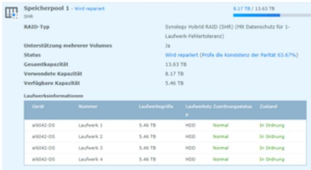
The screenshot shows the 'Speicherpool 1 - Wird repariert' (Storage Pool 1 - Being repaired) status in Synology Storage Manager. The RAID type is Synology Hybrid RAID (SHR) (RAID) with a data protection level of 1. The status is 'Wird repariert (Prüfe die Konsistenz der Parität 63.67%)' (Being repaired (Check parity consistency 63.67%)). The total capacity is 13.63 TB, with 8.17 TB used and 5.46 TB available. Below this, a table lists the drive information for the four drives in the pool.
