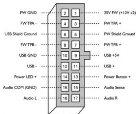
NOTE: View shown here is "top down" of multi-pin connector while connected to motherboard (not "bottom up" after disconnecting from motherboard)
