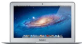
The Apple MacBook Air "Core i5" 1.7 11" (Mid-2012/USB 3.0) features a 22-nm "Ivy Bridge" 1.7 GHz Intel "Core i5" processor (3317U) with two independent processor "cores" on a single chip, a 3 MB shared level 3 cache, 4 GB of onboard 1600 MHz DDR3L SDRAM (which cannot be upgraded after purchase), 64 GB or 128 GB of flash storage, and an "integrated" Intel HD Graphics 4000 graphics processor that shares system memory.
