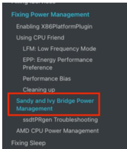
Initializing with OpenCore's setup in the Ivy Bridge section, we recommended users drop their CpuPm and Cpu0Ist to avoid any issues with AppleIntelCPUPowerManagement.kext. But dropping these tables have the adverse affect of breaking turbo boost in Windows. So to resolve this, we'll want to keep our OEM's table but we'll want to add a new table to supplement data only for macOS. So once we're done creating our CPU-PM table, we'll re-add our OEM's CPU SSDTs.
