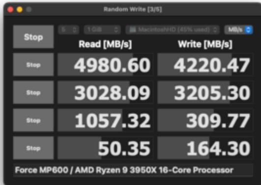
The screenshot shows a benchmark application window titled "Random Write (3/5)". It displays a table of performance metrics for a Force MP600 SSD on an AMD Ryzen 9 3950X 16-Core Processor. The table has columns for "Read [MB/s]" and "Write [MB/s]". Each row includes a "Stop" button and a "1 GB" indicator. The data shows a significant drop in performance from the first to the fifth test.
